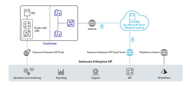
Calls made by an end user at the customer's location are transmitted via the Internet to the cloud telephony provider, from where they are directed via the Enterprise SIP Cloud Trunk to Swisscom and the public telephone network.
