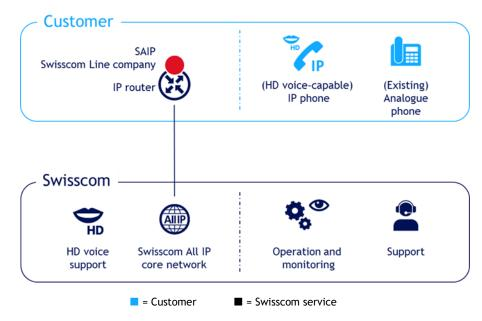
The SAIP is the interface connecting the end devices to the Swisscom IP router at the customer's end.
