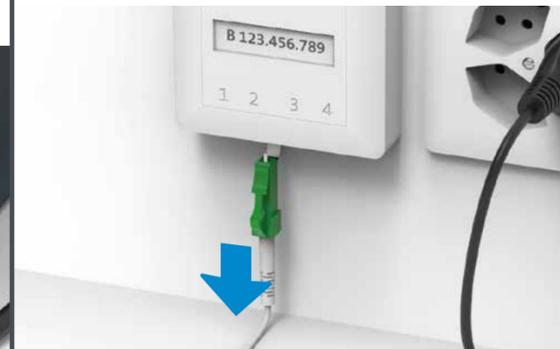
Take note of the slot and pull out the green end of the fibre optic cable.
