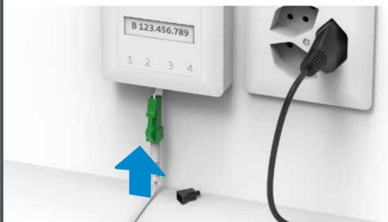
Open the slot at the fibre socket which we have specified by letter (or as in step 2b). This is usually slot 2 (rarely 1).
