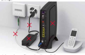
2 Only use the new fibre-optic cable supplied! First connect the new fibre-optic cable to the router and then the fibre-
