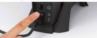
2 First, connect the fibre-optic cable to the router and then the fibre-optic socket (usually slot no. 2, occasionally no. 1).
