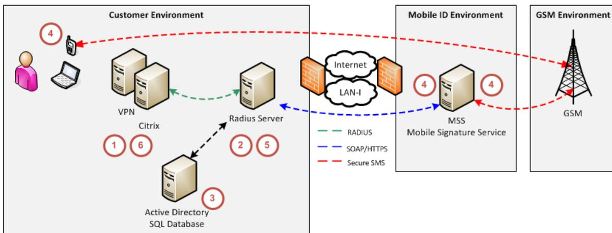
This shows several RADIUS enabled services like VPN and Citrix sending their RADIUS request to a RADIUS server. This RADIUS server will invoke the Swisscom MID web service and provide the answer back to the clients. The RADIUS server may also be connected to an external user store, like Microsoft Active Directory, where the end users details like phone number or credentials are stored. Here the dataflow:
